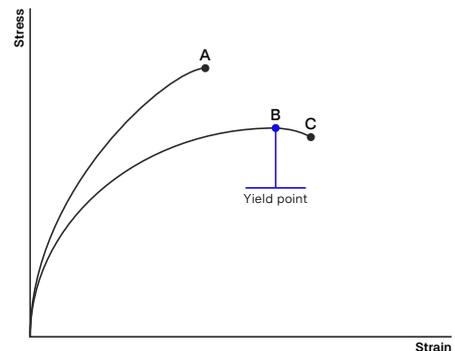
A. Tensile stress at break, elongation at break (no yield point)
